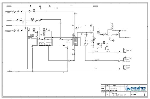
Figure 1. Simplified P&ID of the NextGen pilot plant where MBR system is applied.
