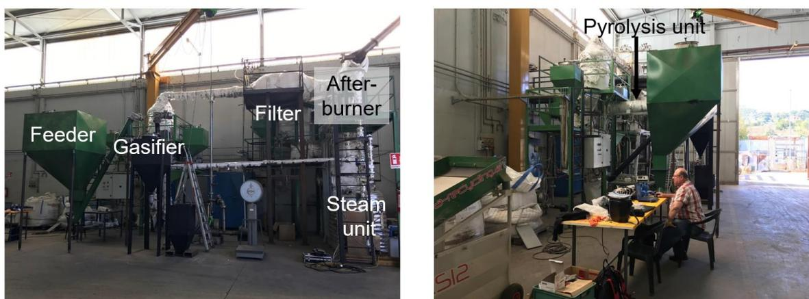
Fig. 2: Front and side view of the thermal treatment units (picture owner: CTU)
