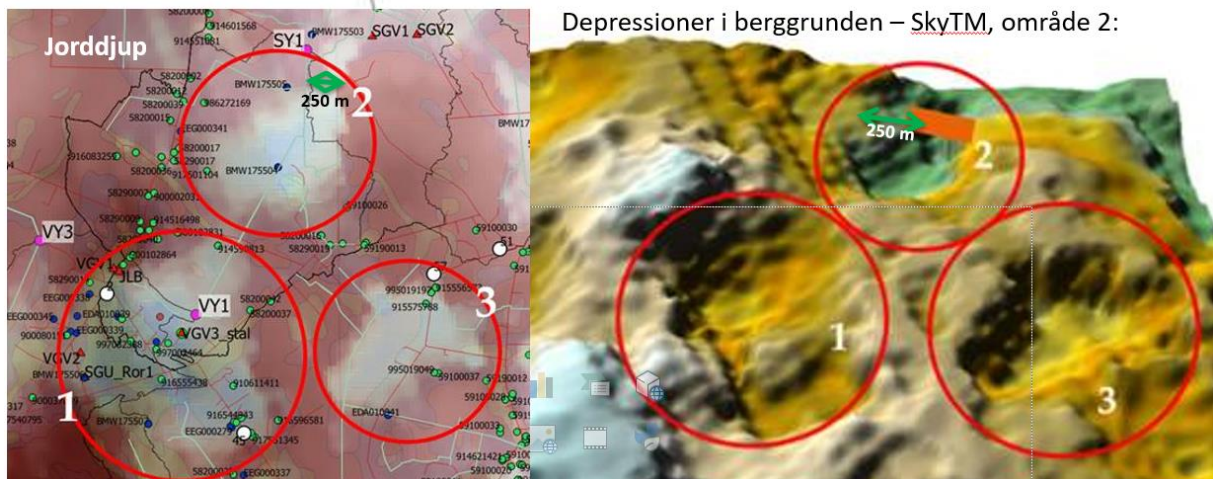
Figure 2. The use of electromagnetic Sky-TM measurements from helicopter for finding ground water pounds. The area n° 2 is the area shown in figure 1 and shows a so-called depression in the rock that most probably is filled mainly with sand and therefore should be a good area for underground storage of water.
