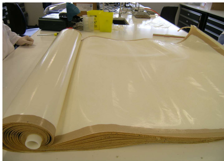
Fig. 3 Spiral wound RO membrane element.
