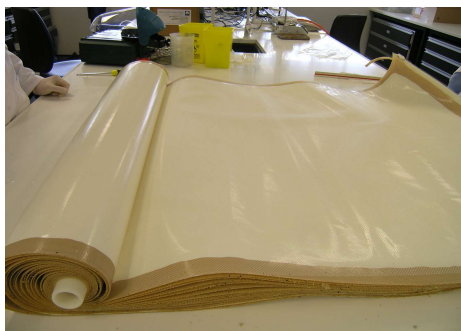
Fig. 3 Spiral wound RO membrane element.
