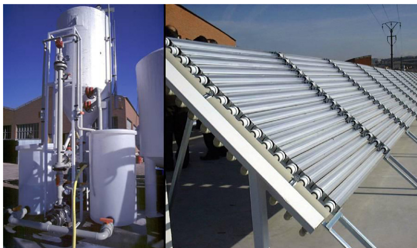
Fig. 15. Photographs of solar detoxification demonstration plant constructed in “SOLARDETOX” project at HIDROCEN (Madrid, Spain). Left: TiO 2 separation system. Right: compound parabolic collector.
